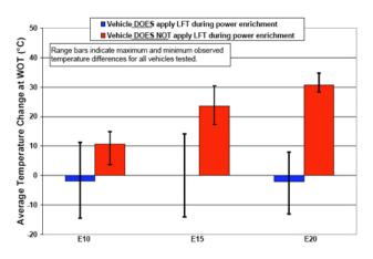
Panel B. Increase in catalyst temperature for E10, E15, and E20 fuels compared to E0 for vehicles operated at wide-open throttle (WOT) open-loop conditions. 43% of tested vehicles (red bars) experienced higher catalyst temperatures; the rest of the tested vehicles (blue bars) were able to maintain stable catalyst temperatures. Source: Figure 3.5 in the DOE (2009) report.
