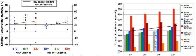
**Panel D.** Exhaust temperature increased for all non-road engines operated on ethanot piends. Lett panet. Exhaust temperature increase for all small non-road engines tested in the new and full-useful-life (full-life) condition with ethanol blends, as compared to E0 baseline. Source: Figure 3.6 in the DOE (2009) report. **Right panel.** Exhaust port temperature for pilot study engines at hottest condition versus ethanol blend level. Source: Figure 3.15 in the DOE (2009) report.
